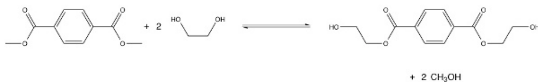
Scheme 1. Transesterification reaction between dimethyl terephthalate and ethylene glycol.
