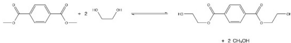
Scheme 1. Transesterification reaction between dimethylterephthalate and ethylene glycol.
