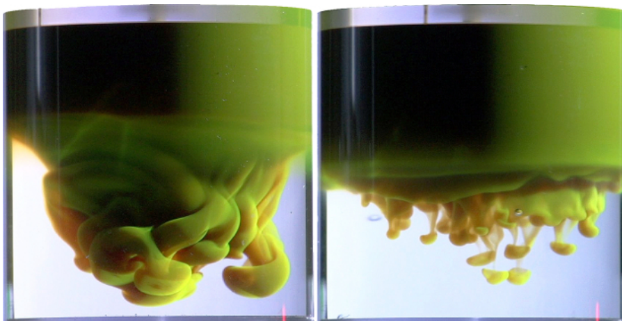
Figure 1: Qualitative effect of rotation on the Rayleigh-Taylor Instability. The image on the left hand side is of the Rayleigh-Taylor instability developing in a non-rotating system. The instability develops in time, forming large vortices that transport the 'denser' (green) fluid downwards. The image on the right hand side is of the same fluids, and therefore the same gravitational/magnetic instability, but here the system is rotating. The effect of the rotation can be seen to restrict the size of the vortices that form and inhibit the bulk vertical transport of fluid. The times shown are 1.92 s and 3.52 s after initiation on the left hand side and right hand side respectively. The tank diameter is 90 mm, and the rotation rate in the right hand image was 2.38 rad s -1 . Please click here to view a larger version of this figure.
