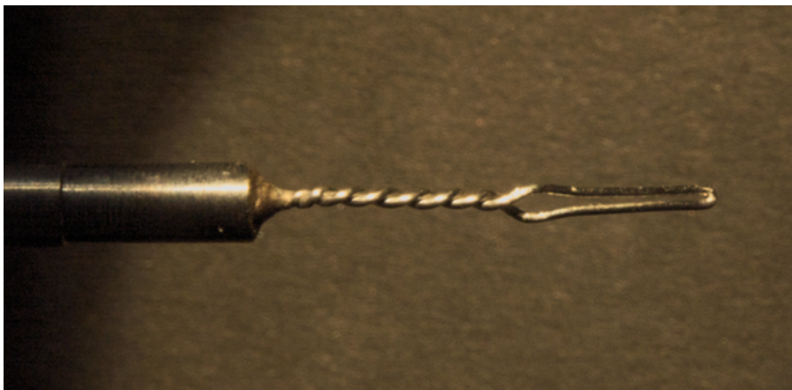
Figure 1: Platinum Loop. The platinum wire loop mentioned in protocol step 1.4. Platinum is a metal that can be bent without producing splinters, and it does not stick to biological material. Please click here to view a larger version of this figure.
