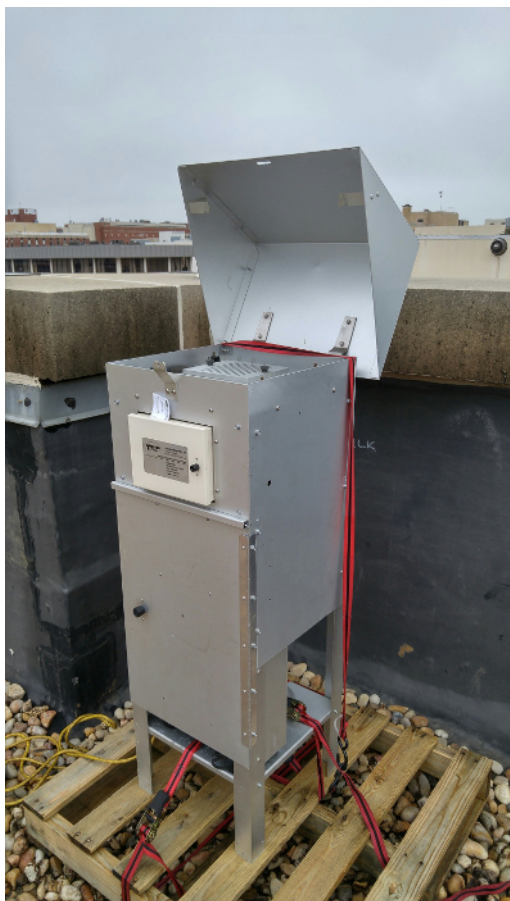
Figure 1. The high volume total suspended particles (TSP) sampler. The picture shows the TSP sampler installed in a roof in an urban area to collect ambient particles. Please click here to view a larger version of this figure.
