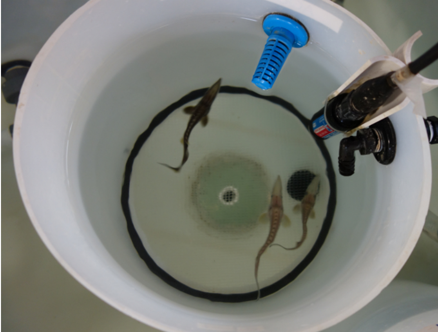
Figure 2. Polyethylene tank. A 19 L domed bottom polyethylene tank showing the overflow drain (top, with screen insert; 1.3.1; 5.6.1), slurry water inlet (right elbow; 1.3.2), pump outlet (center bottom; 1.3.3), pump inlet (off-center bottom; 1.3.4), OBS probe and clamp (4.1), and bottom screen (black ring on bottom; 5.6.1). Please click here to view a larger version of this figure.
