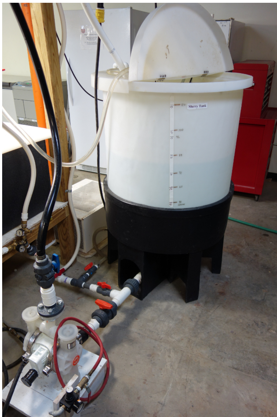
Figure 4. Slurry tank. Cone-bottom slurry tank with cover and poly stand. Slurry water temperature is controlled by water chiller located on the floor left of the stand. The tank is connected to an air operated double-diaphragm pump (left foreground) to provide slurry to each aquarium (2.2). Please click here to view a larger version of this figure.
