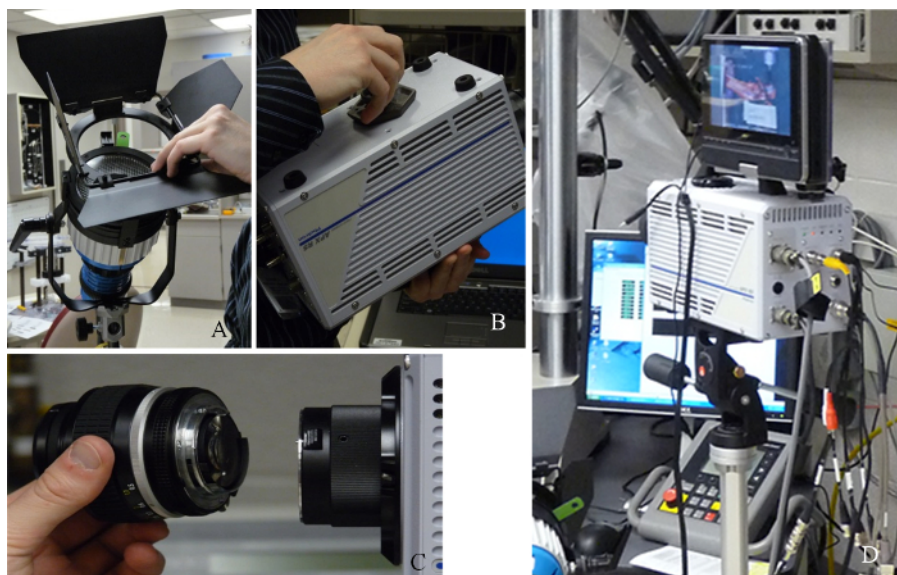
Figure 3: Lighting and Cameras Installation. (A) Setting up lamps and shields; (B) Attaching the high-speed camera to the tripod; (C) Installing the lens to the camera unit; (D) Connecting the camera to the computers. Please click here to view a larger version of this figure.
