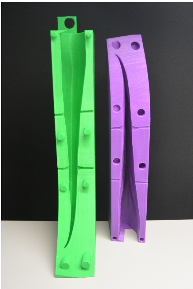
Figure 3: Mold. The mold used to create the flexible portion of the robotic flipper is created from the scanned flipper specimen. The mold has two parts: an upper (purple) and a lower section (green) that are aligned with male and female posts, respectively. The robot skeleton ( Figure 4 ) is aligned inside the mold before the silicon mixture is poured into the mold. Please click here to view a larger version of this figure.
