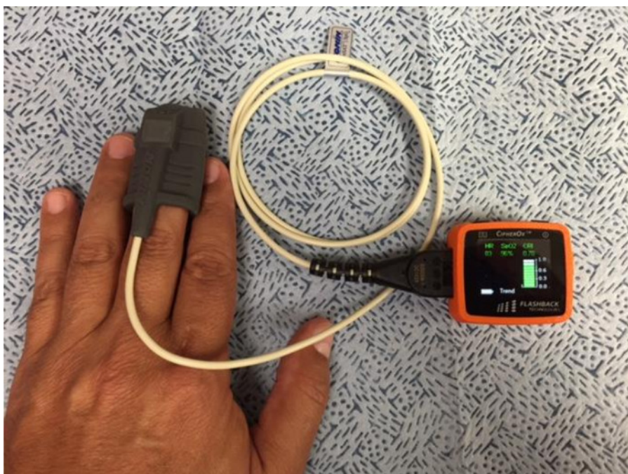
Figure 2: Compensatory Reserve Monitoring Device. The device consists of a noninvasive finger pulse oximeter that transmits pulse oximeter and waveform data via a USB connection to a compensatory reserve monitor. The monitor unit contains an algorithm which calculates a value for compensatory reserve known as the Compensatory Reserve Index (CRI) 1,12 . Data are recorded at each heart beat and displayed on the monitor and stored on a memory card. Please click here to view a larger version of this figure.
