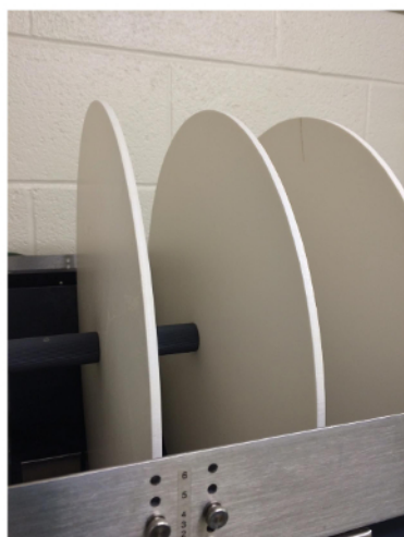
Figure 2: The Rotarod Apparatus. The Rotarod test is a standard neurobehavioral assay in which mice are trained to run on a rotating rod and are timed for how long they can stay on the rod as it slowly speeds up. The rod is suspended above a cage floor, and mice naturally try to stay on the rod to avoid falling to the ground. The drop from the rod to the base of the instrument causes no injury to the mice. A) A standard Rotarod apparatus consists of a motor-driven rod with constant or accelerating speeds. B) Panels divide the rod into separate lanes, each suited for an individual animal. A total number of 4 mice can be tested during each trial. C) The rod is 1.18 in. (about 3 cm) in diameter, and its surface is knurled, allowing the mice to get a better grip. The fall of the mouse is precisely tracked by a photo beam that automatically records the amount of time spent on the rod. The experimental data is recorded in a computer after the mice have all fallen from the rod. Please click here to view a larger version of this figure.
