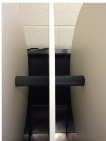
Figure 2: The Rotarod Apparatus. The Rotarod test is a standard neurobehavioral assay in which mice are trained to run on a rotating rod and are timed for how long they can stay on the rod as it slowly speeds up. The rod is suspended above a cage floor, and mice naturally try to stay on the rod to avoid falling to the ground. The drop from the rod to the base of the instrument causes no injury to the mice. A) A standard Rotarod apparatus consists of a motor-driven rod with constant or accelerating speeds. B) Panels divide the rod into separate lanes, each suited for an individual animal. A total number of 4 mice can be tested during each trial. C) The rod is 1.18 in. (about 3 cm) in diameter, and its surface is knurled, allowing the mice to get a better grip. The fall of the mouse is precisely tracked by a photo beam that automatically records the amount of time spent on the rod. The experimental data is recorded in a computer after the mice have all fallen from the rod. Please click here to view a larger version of this figure.
