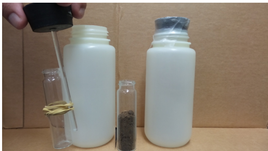
Figure 1. Incubation container for conducting sequential fumigation incubation procedure for labile organic C and potential C turnover rate determination. On the left is the Nalgene bottle, vial suspended from a stopper rod to contain NaOH, and a vial containing 30 g of soil shown separated for demonstration purposes. The container on the right has the soil and the stopper rod positioned within the Nalgene bottle with Parafilm along the top as would be done during incubation. Please click here to view a larger version of this figure.
