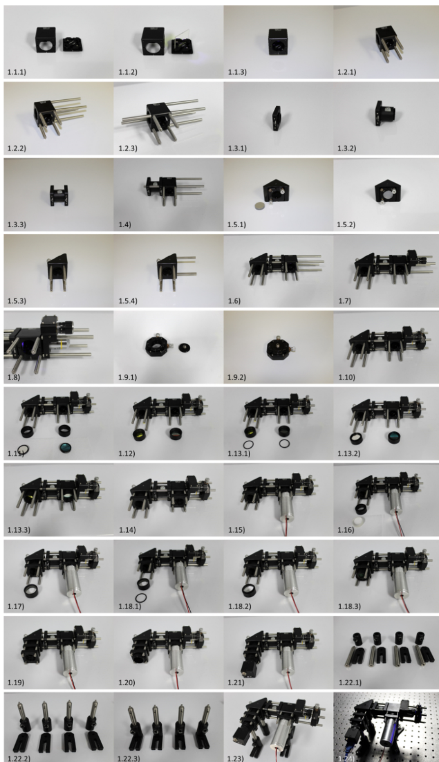
Figure 2: Assembly of the high-resolution fluorescence microendoscopy modality. The high-resolution fluorescence microendoscopy modality can be constructed by building a shell of 1.0 inch diameter-sized components, with special care taken in handling the dichroic mirror, objective lens, excitation/emission filters, and tube lens. Glass surfaces of these components must be carefully handled using lens paper. Please click here to view a larger version of this figure.
