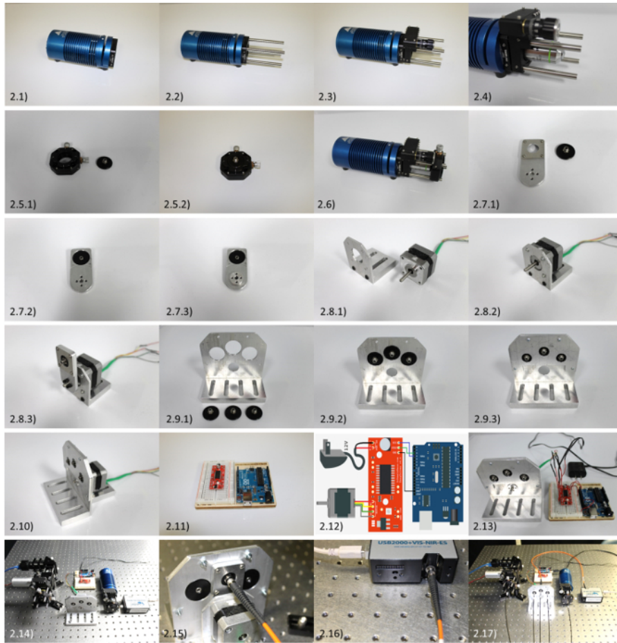
Figure 3: Assembly of the sub-diffuse reflectance spectroscopy modality. The sub-diffuse reflectance spectroscopy modality can be constructed using a basic tungsten-halogen lamp coupled to an objective lens to focus light through the 200 \mu\text{m} multimode delivery fiber, and a spectrometer. Additionally, a custom-built motorized optical switch can be constructed within the lamp-fiber-spectrometer path to switch between each SDS. Investigators using multiple spectrometers to acquire from multiple SDSs can bypass the optical switch component. Please click here to view a larger version of this figure.
