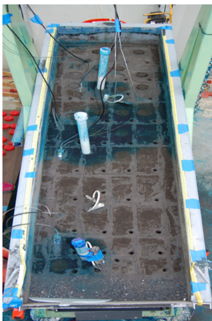
Figure 4. Top view of lysimeter. This view shows the dyed surface of layer 2 (10 cm deep). Grids drawn on the soil surface to aid sampling are also visible, along with core holes regions at each voxel after microbiological sample collection.
