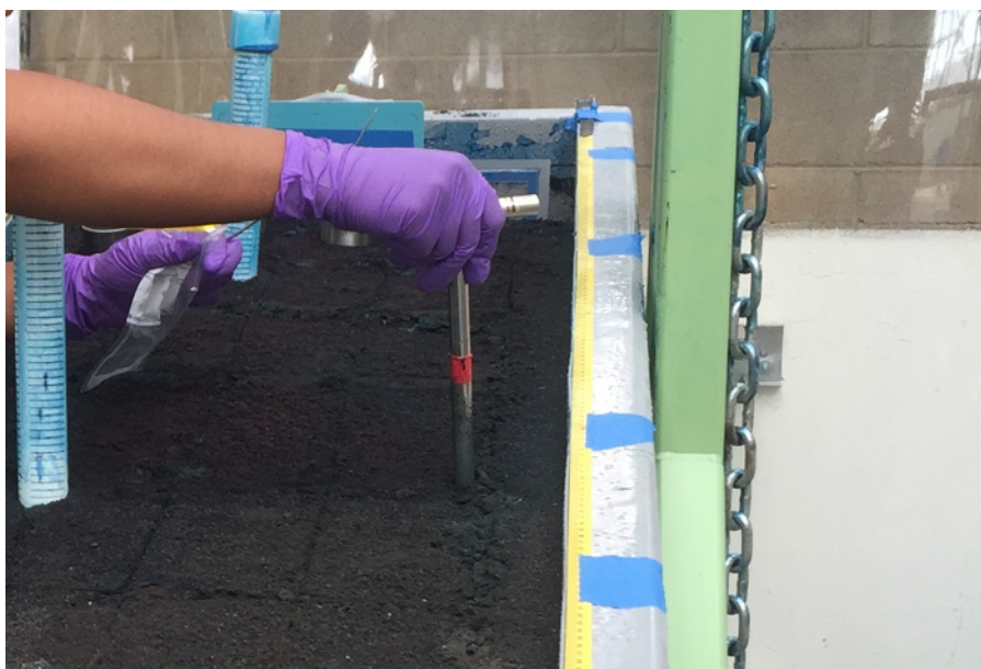
Figure 5. Microbiology sample collection. A small handheld corer of 20 cm x 1 cm, sterile bags, and spatula is shown here during microbiological sampling. Please click here to download this file.
