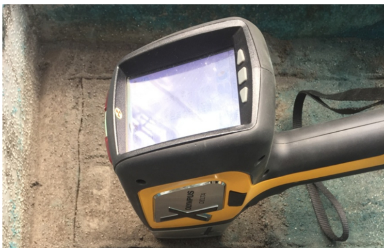
Figure 7. Portable X-ray Fluorescence Spectrometer. Handheld pXRF positioned on surface of a voxel. Measurements were recorded at three different locations on the surface of each voxel and then averaged.
