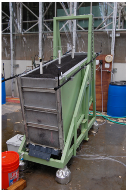
Figure 1. Side-view of lysimeter. View of lysimeter from the seepage face. Also visible are three sensor regions (white PVC tubes) along the slope and sprinkler system at the four corners.
