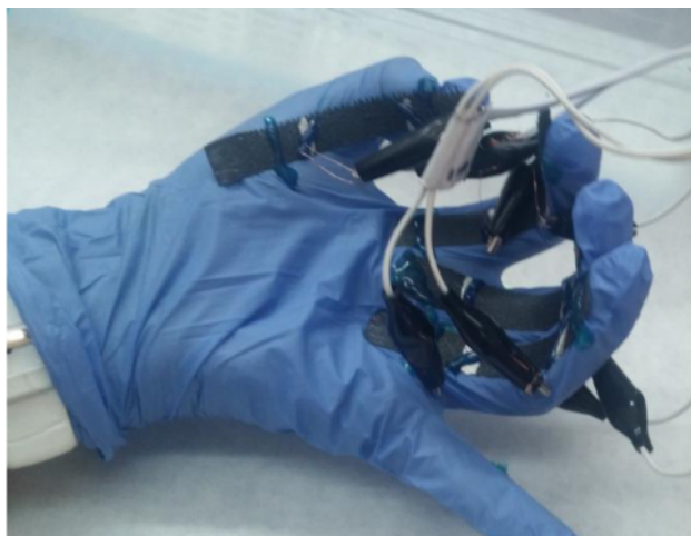
Figure 2. Location of f-GNP/glass fiber bands on the internal surface of the fingers of a nitrile glove to monitor fingers bending. Once the glass fiber fabric has been coated and dried, bands 10 mm in width are cut and attached on the different fingers of a glove with the aim of monitoring the finger bending and corroborate the viability of the protocol described above. Please click here to view a larger version of this figure.
