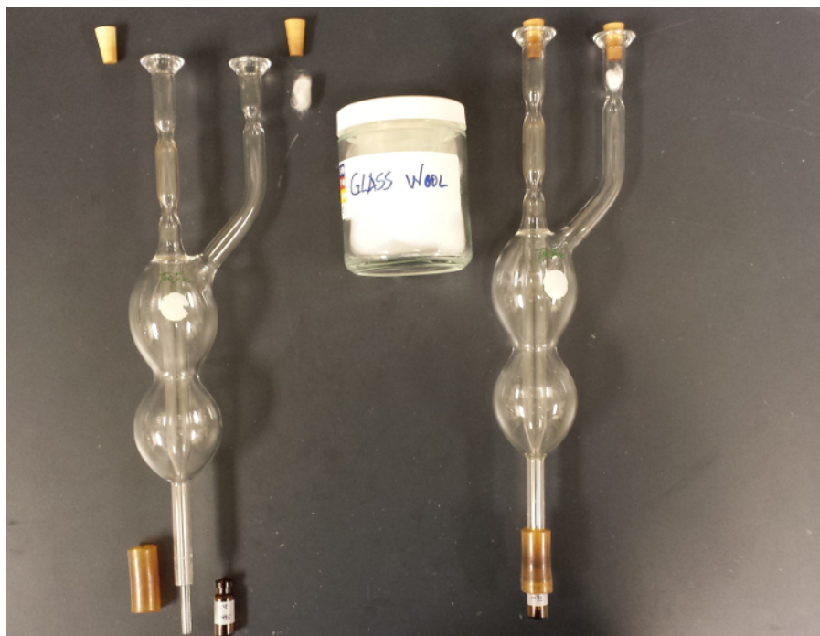
Figure 2: Vial attachment to condenser. Photo showing the location of the glass wool plug and the attachment of a GC vial to the condenser with silicone tubing. Please click here to view a larger version of this figure.
