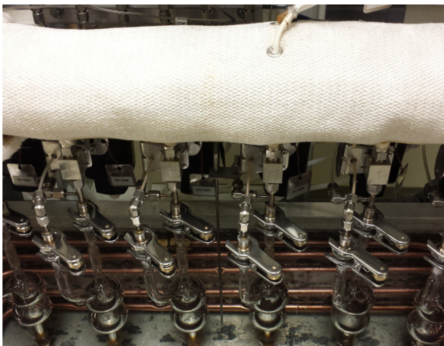
Figure 4: Liquid receiver attachment. Photo showing the attachment of liquid receivers to the product line. Please click here to view a larger version of this figure.
