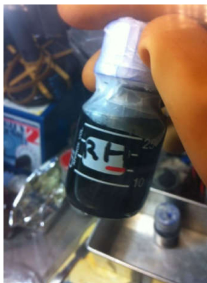
Figure 2: After all the metallic Li had dissolved in \text{TPB}(\text{THF})_{24.7} , the colors of \text{Li}_x\text{TPB}(\text{THF})_{24.7} ranged from light blue (for x = 1 ) to very dark blue (for x = 4 ). A lighter color indicates a lower concentration of solvated electrons in the \text{TPB}(\text{THF})_{24.7} solution. This photograph shows a solution of \text{Li}_3\text{TPB}(\text{THF})_{24.7} for x = 3 which has a dark blue color. Please click here to view a larger version of this figure.
