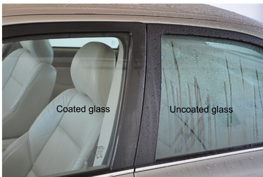
Figure 4. Demonstration of Hydrophilic Coating (2). Driver's seat window of an automobile was coated with nanoparticles while rear passenger window was uncoated. When both windows were sprinkled with a water sprayer, coated surface did not form water droplets. Please click here to view a larger version of this figure.
