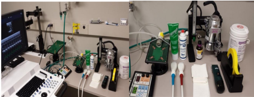
Figure 1: Animal Cardiac Ultrasound Laboratory. The laboratory is equipped with the small-animal-dedicated ultrasound machine with high frequency (30 MHz and 40 MHz) transducers (MS 400 and MS 550D), isoflurane diffuser, animal platform, temperature and heart rate monitor, 1% to 1.5% isoflurane mixed with 1 L/min 100% O 2 , nose cone and tubing connected to isoflurane diffuser and 100% O 2 , hair razor, ultrasound gel, electrode gel, adhesive tapes, and paper towels. Please click here to view a larger version of this figure.
