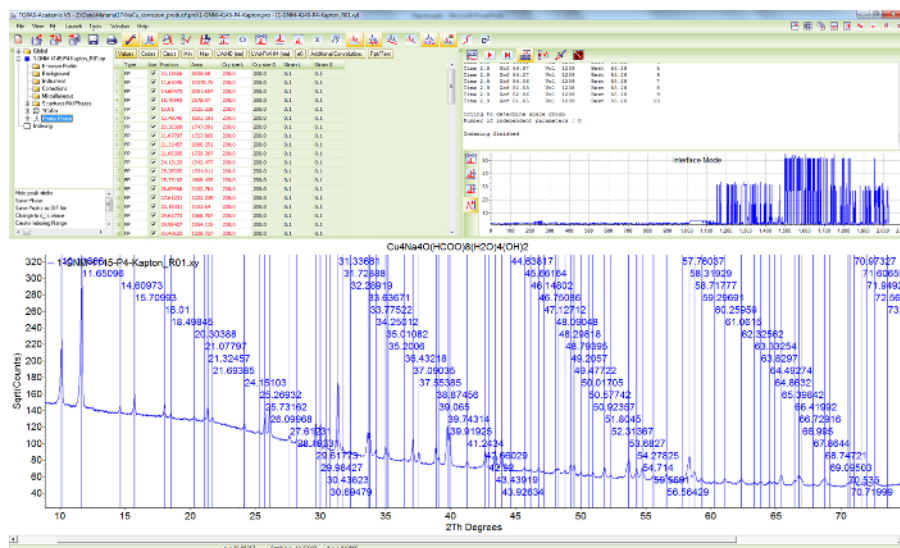
Figure 10. Peak search for sample 1. Screen shot showing the scattered X-ray intensities of \text{Cu}_4\text{Na}_2\text{O}(\text{HCOO})_8(\text{OH})_2 \cdot 4\text{H}_2\text{O} and the results of the automatic peak search algorithm using first and second derivatives of Savitzky-Golay smoothing filters. Please click here to view a larger version of this figure.
