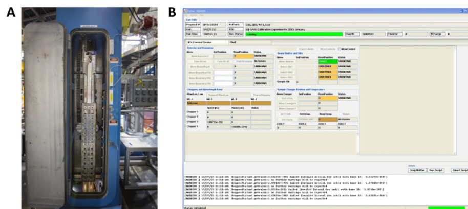
Figure 3. Standard EQ-SANS experiment environments. (A) Sample booth, and (B) control software at the beam line. Please click here to view a larger version of this figure.
