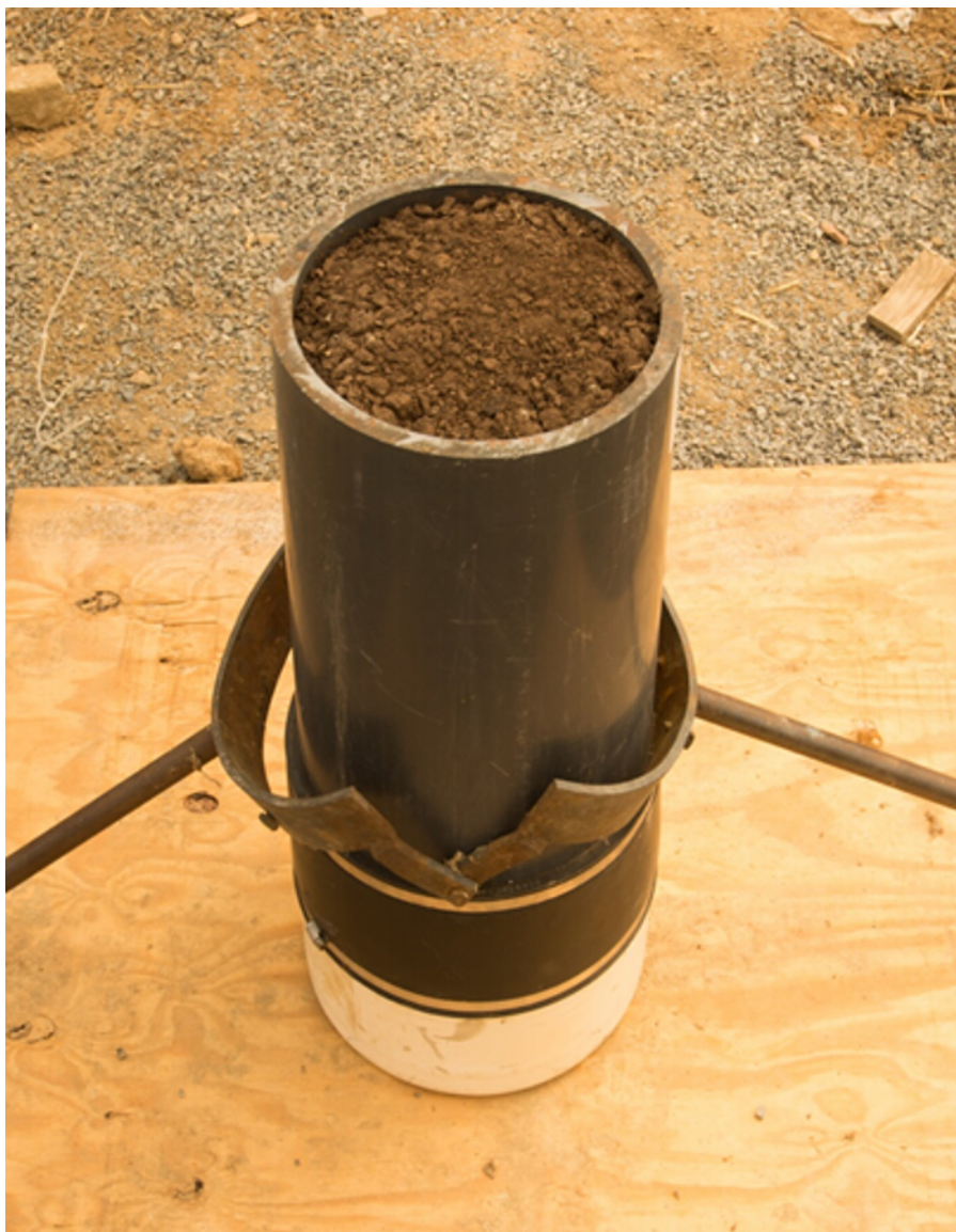
Figure 2: Custom lifting scissors. Custom lifting scissors allow two people to lift and move heavy soil core lysimeters. Please click here to view a larger version of this figure.
