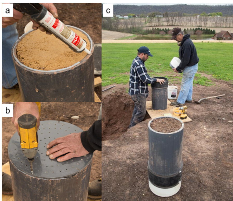
Figure 6: Installing bottom onto lysimeter. (a) Putting a ring of caulk on cleaned rim of lysimeter. (b) Fastening perforated disk onto lysimeter with stainless steel screws. (c) Putting cap on lysimeter and fastening tight with flexible coupling. Please click here to view a larger version of this figure.
