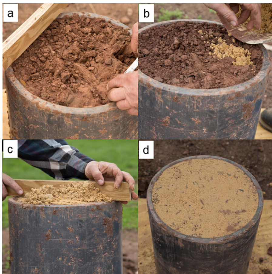
Figure 5: Preparation of lysimeter bottom for perforated plate and cap. (a) Leveling bottom and removal of protruding stones. (b) Filling voids with sterile sand. (c) Leveling sand. (d) Cleaned column with level sand. Please click here to view a larger version of this figure.
