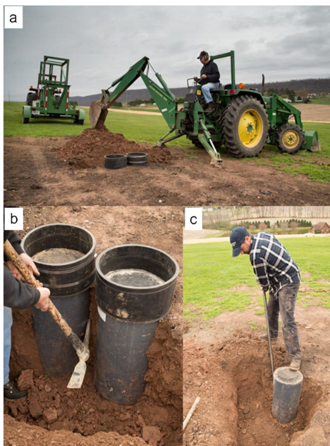
Figure 4: Preparation for removal of soil columns. (a) Hole being dug along-side of columns. (b) Soil being picked away from columns (note lysimeters protected from external soils with PVC cover and flexible coupling). (c) Soil-to-soil interface being broken with a digging bar. Please click here to view a larger version of this figure.
