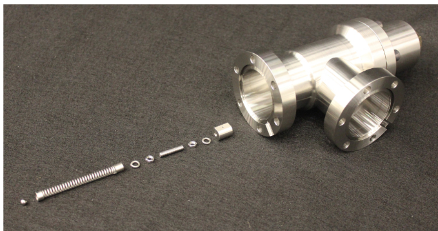
Figure 5: Elements of the Spring Transport Mechanism. In order of assembly (from right to left), the parts shown are: valve, thread adapter, lock-washer, nut, cut 8-32 stud, nut, lock-washer, ball-holder/spring assembly, and 4.5 mm rotor.
