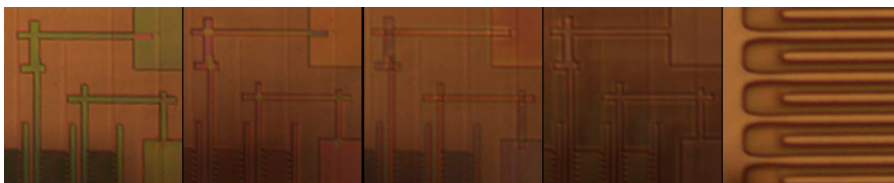
Figure 3: Sample LOR Development Process. Images of the same area of a device as the LOR is developed. The picture on the far left was taken under a microscope after the initial 25 sec development time. The pictures that follow are a sampling of the changes through the iterative process. The final picture is a close-up of the finer features on the device after LOR development to show the clean edges and the exposure of the underlying substrate. Please click here to view a larger version of this figure.
