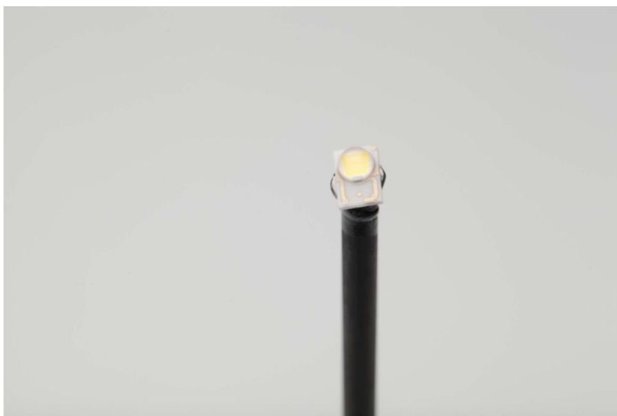
Figure 2. Specimen prepared for CT. LED mounted on carbon fiber bar in slanted position. Please click here to view a larger version of this figure.
