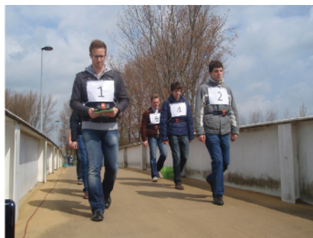
Figure 5. (A) The Eeklo footbridge and (B) synchronized walking of six participants (this figure has been modified from [3]). Please click here to view a larger version of this figure.
