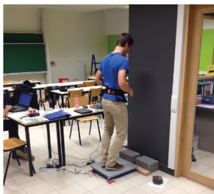
Figure 4. Configuration setup for the laboratory experiments involving human rhythmical experiments. Please click here to view a larger version of this figure.
