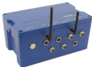
Figure 3. Wireless triaxial Geosig sensors 5 applied to register the structural accelerations. Please click here to view a larger version of this figure.
