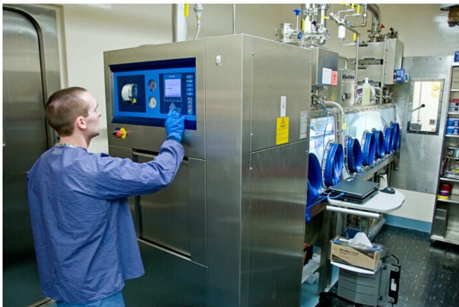
Figure 3. Interlocking Double-door Autoclave Attached to the Class III BSC. A researcher is selecting a pre-programmed autoclave cycle to ensure the contents within the autoclave chamber are noninfectious when the outer door is eventually opened. The door located nearest to the researcher cannot be opened until a full sterilization cycle has been completed. Biological indicators inside the autoclave chamber will be analyzed to determine agent inactivation after the sterilization process (reproduced from 5 ). Please click here to view a larger version of this figure.
