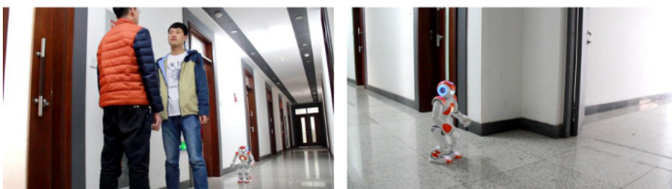
Figure 5. Telepresence Control Experiment of Walking Toward the Staircase Following the Exit Sign. Please click here to view a larger version of this figure.
