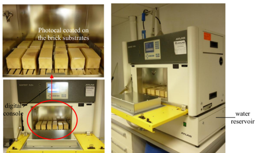
Figure 3. Weathering Chamber. The commercial form of the Suntest XLS+ weathering chamber contains a stainless steel hood inside which the nanocoated samples are placed. The water reservoir is placed beneath the hood which is the source of the water to be sprayed inside the hood. Please click here to view a larger version of this figure.
