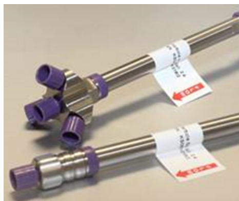
Figure 1. An image of Active Flow Technology column compared to a conventional column. The AFT column is fitted with a four port outlet fitting that houses the annular frit enabling peak sampling across the radial cross section of a sample band. Please click here to view a larger version of this figure.
