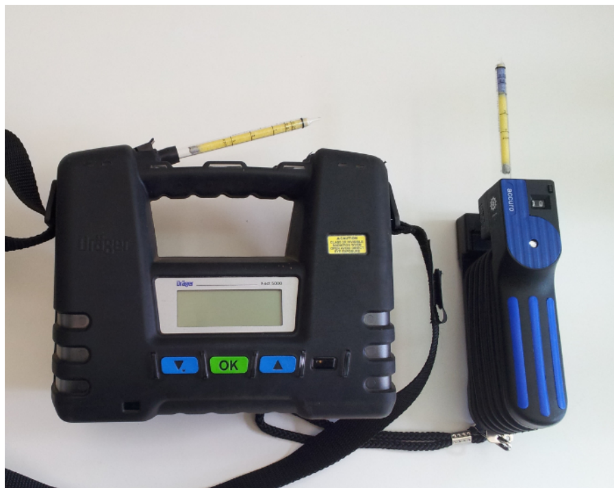
Figure 4: Indicator tubes with pump dispenser and hand pump. Right side: hand pump (stroke counter, window for pump control with white spot) with used indicator tube; left side: pump dispenser (control display, control buttons) and new indicator tube (0.25-3 ppm). Original filling of indicator tube has a yellow color. Reaction with ammonia results in a change to purple color, color front is dislocated within the scale. Ammonia concentration values are obtained by reading the scale.
