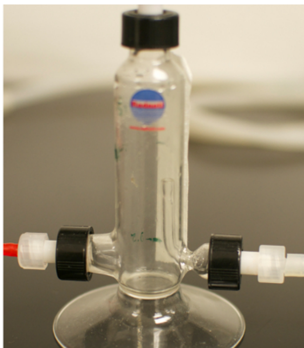
Figure 3. Flow Damping Chamber. Flow damping chamber schematic indicates intended flow direction and connection. Air release valve is opened, outlet valve is closed, and fluid fills the chamber to desired PI level. Upon opening of outlet valve and closing of air release valve, flow resumes and fluid levels within the chamber maintains levels. Please click here to view a larger version of this figure.
