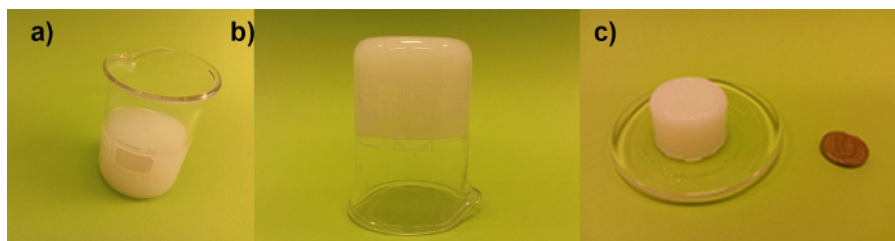
Figure 4: Gelation in heptane. (a and b) organogel of gelator 1 in heptane (5 mg/ml). (c) Gel removed from the beaker.
