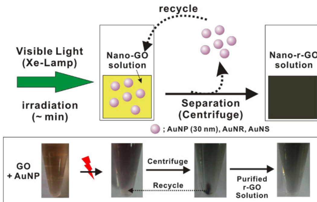
Figure 1. Reaction scheme for r-GO synthesis. Schematic description of r-GO synthesis using plasmonic nanoparticle and visible light. (Reprint with the permission from ref. 13) Please click here to view a larger version of this figure.
