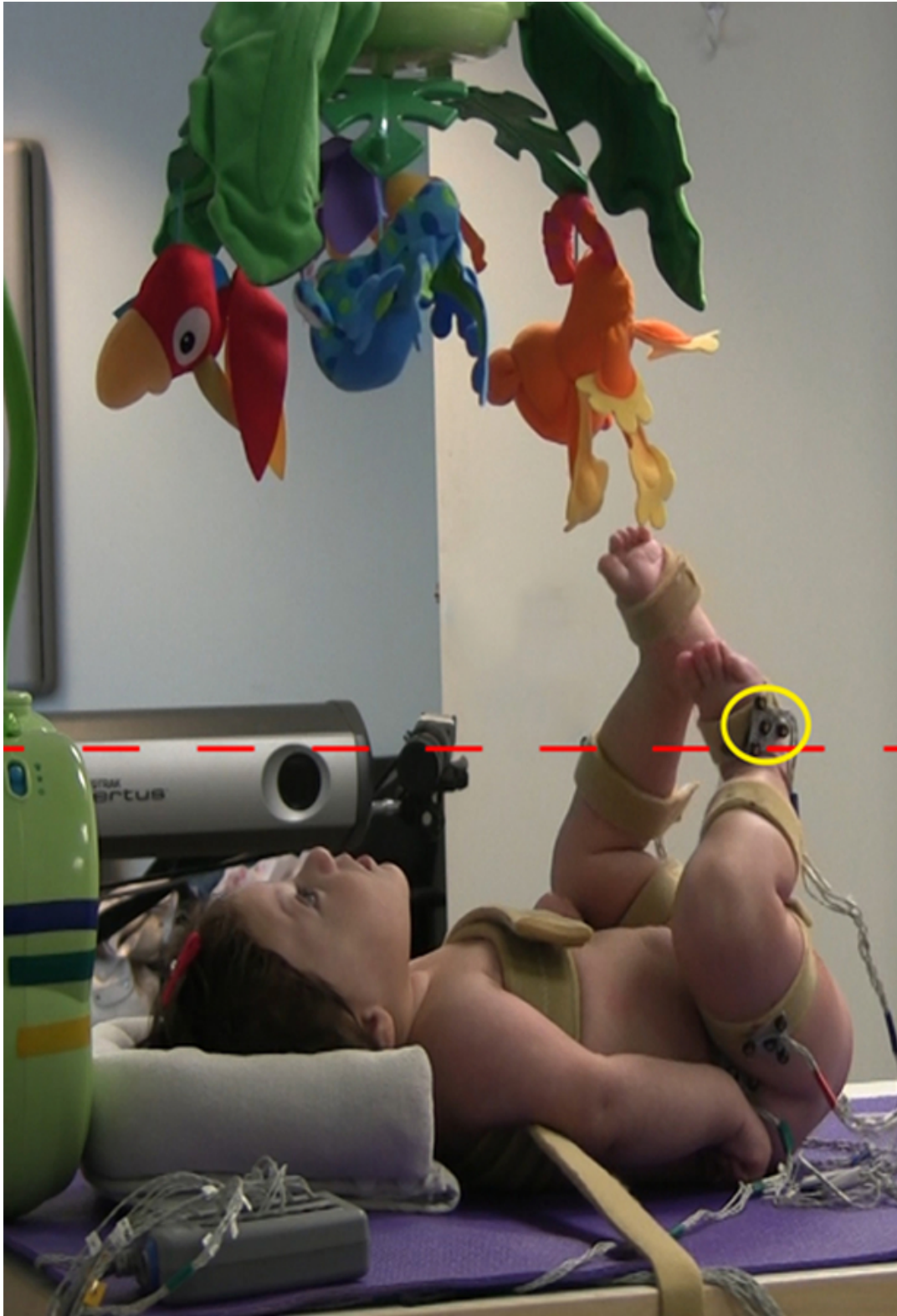
Figure 1: Infant kicking-activated mobile task. The center light-emitting diode (LED) attached to the rigid body of each foot (yellow circle) activates the mobile when it crosses the virtual threshold (red dashed line). Re-printed with permission from Sargent et al. 3
