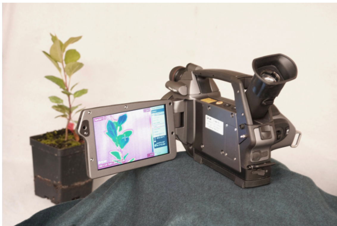
Figure 1. High-resolution Infrared Radiometer. The model illustrated is a FLIR SC-660 Infrared Video Camera.
