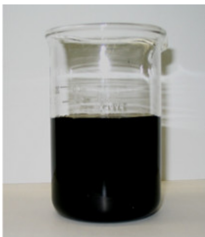
Carbon Nanotubes After Sonication (six months)
