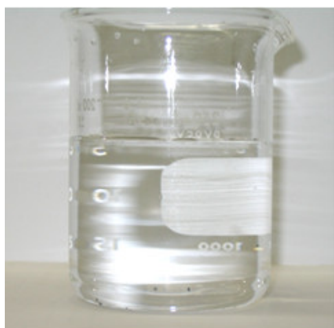
Carbon Nanotubes Before Sonication
