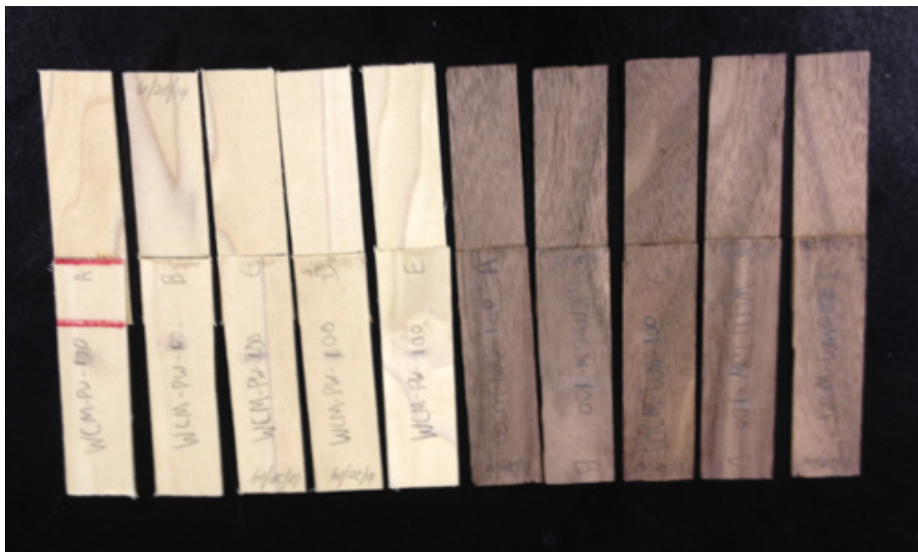
Figure 2. Bonded wood specimens set aside for conditioning (temperature of 22 - 23 °C and relative humidity of 50 - 60%). Left 5, poplar; Right 5, walnut. The bonded area (25.4 x 25.4 mm or 1.0" x 1.0") is shown between the red lines at the most left pair. Please click here to view a larger version of this figure.
