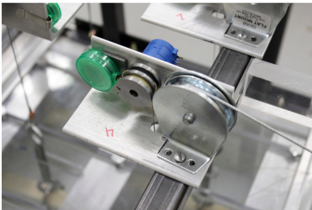
Figure 3. String potentiometer assembly of the testing apparatus. Please click here to view a larger version of this figure.
