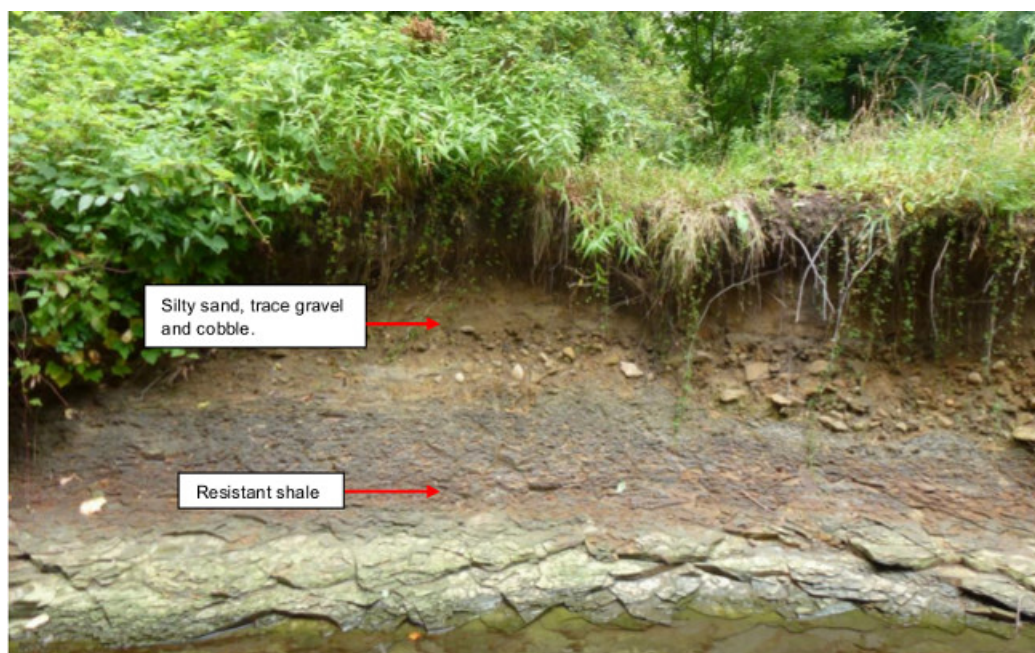
Figure 4. Bank Material Metric. Adjustments can be made based on the erodibility of the material. A mixture of material, as shown in the figure is often found in stream systems so an average score would be more appropriate.
