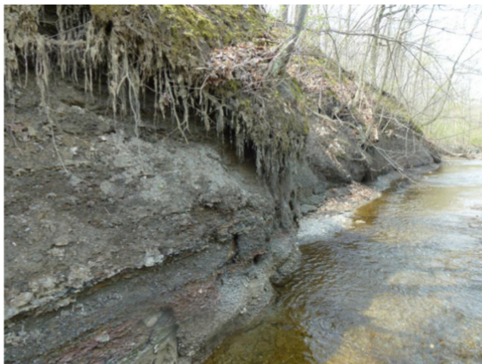
Figure 11. Shale Wall. The weathered shale wall that was unable to be assessed with the original BEHI protocol because bedrock automatically receives a very low BEHI score; however, after completing the modified BEHI protocol, this streambank ranked extreme.
