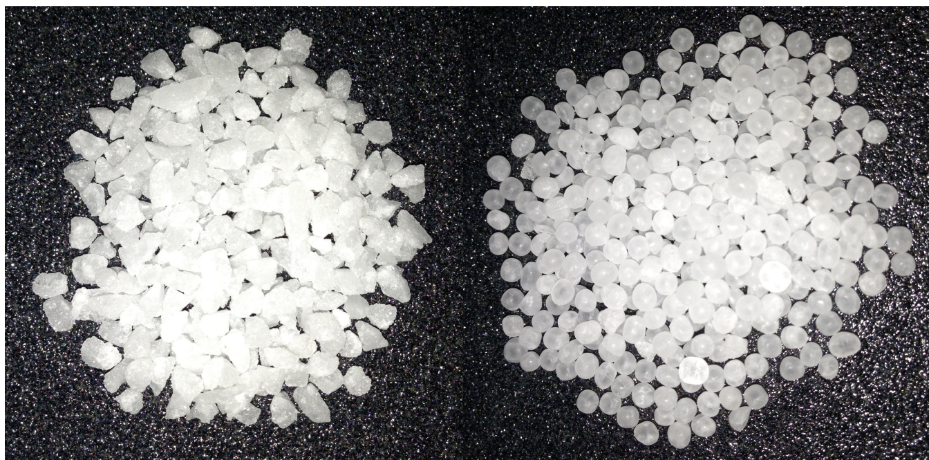
Figure 4. Morphology of the NaCl Grains (Left: Angular 2–2.36 mm; Right: Spherical 1.4–1.7 mm).
