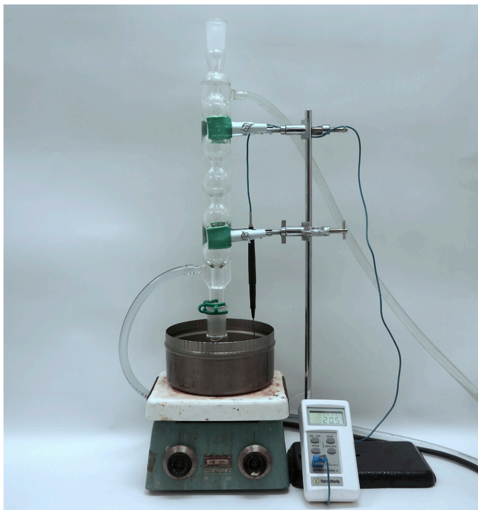
Figure 1. An experimental setup for synthesis of primary iron oxide core/gold shell nanoparticles. A round-bottom flask is connected to a condenser. The reaction is carried out in an oil bath under temperature monitoring by a thermometer.
