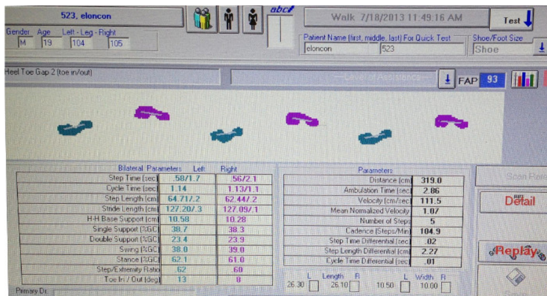
Figure 7: Example data produced by gait analysis system. The top is the foot pressure on the mat and the bottom has all the kinematic measures.
