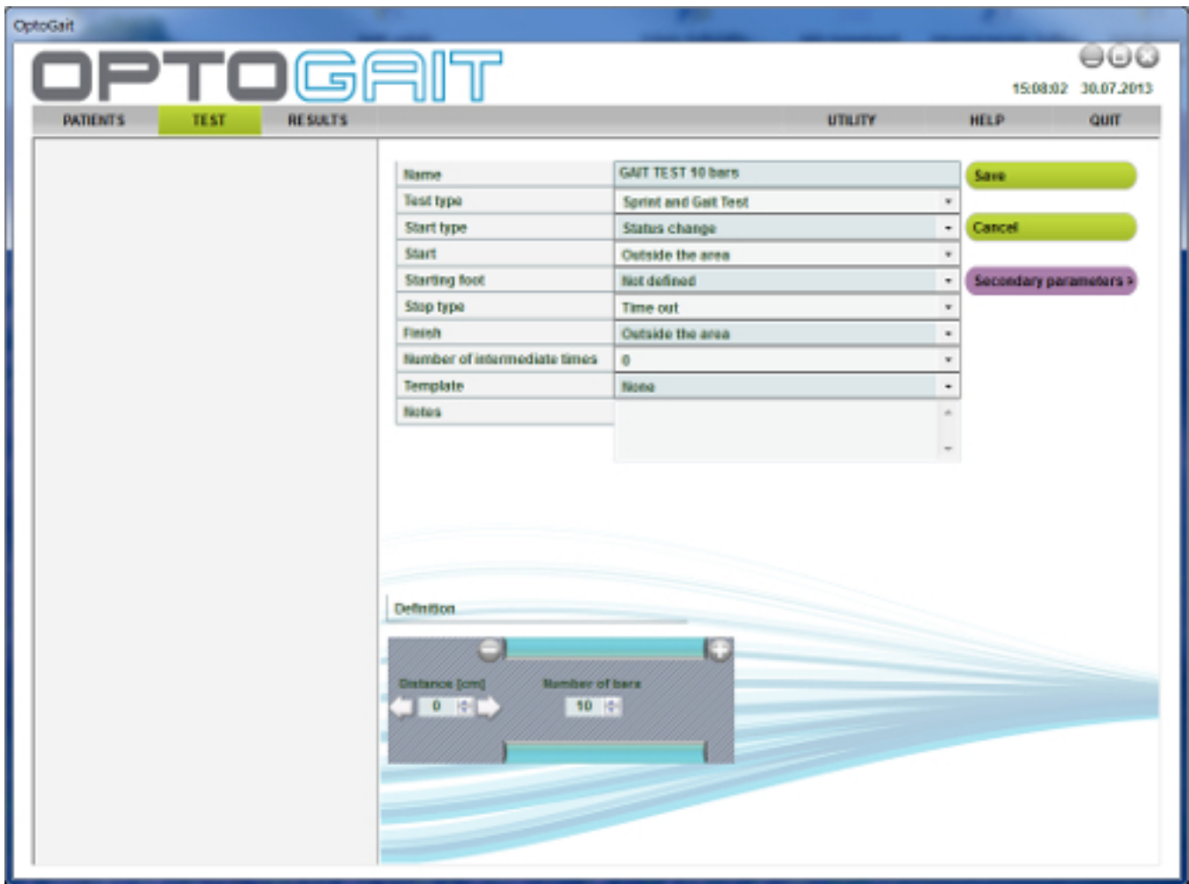
Figure 2. Standard settings for a gait test with 10 bars, as described in the present protocol. These settings have to be defined when the photoelectric system is used for the first time. In this protocol the starting foot is not defined. The system starts measuring when the patient enters the recording area and stops measuring when the patient leaves the measuring units. Please click here to view a larger version of this figure.
