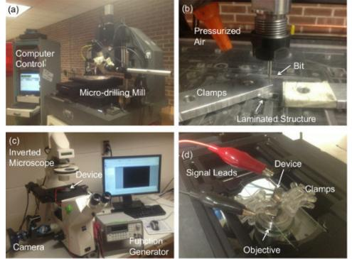
Figure 2. a) Computer-controlled micro-drilling machine. b) Laminated structure is immobilized on the stage with clamps. Pressurized air is used to blow debris off the end mill. c) Microdevice experiments are conducted with a microscope, CCD camera, function generator and computer for data acquisition. d) Close-up view of microdevice clamped onto a glass slide on the microscope stage. AC electrical signal from the function generator is applied to the device through the copper leads.
