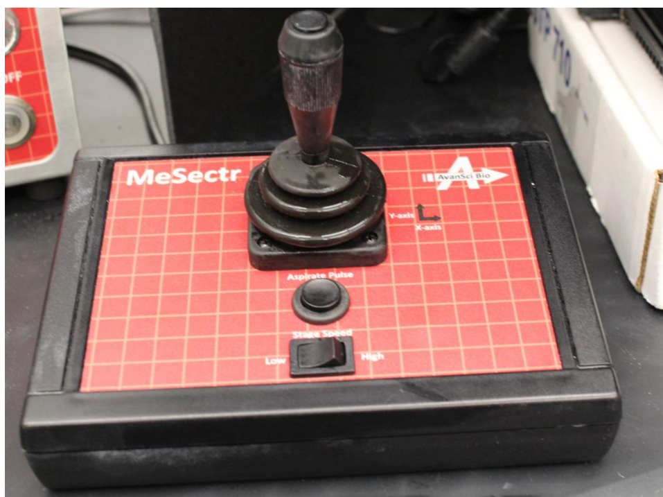
Figure 3. Closer view of joystick. The joystick, “aspirate pulse” and “stage speed” buttons shown. Please click here to view a larger version of this figure.
