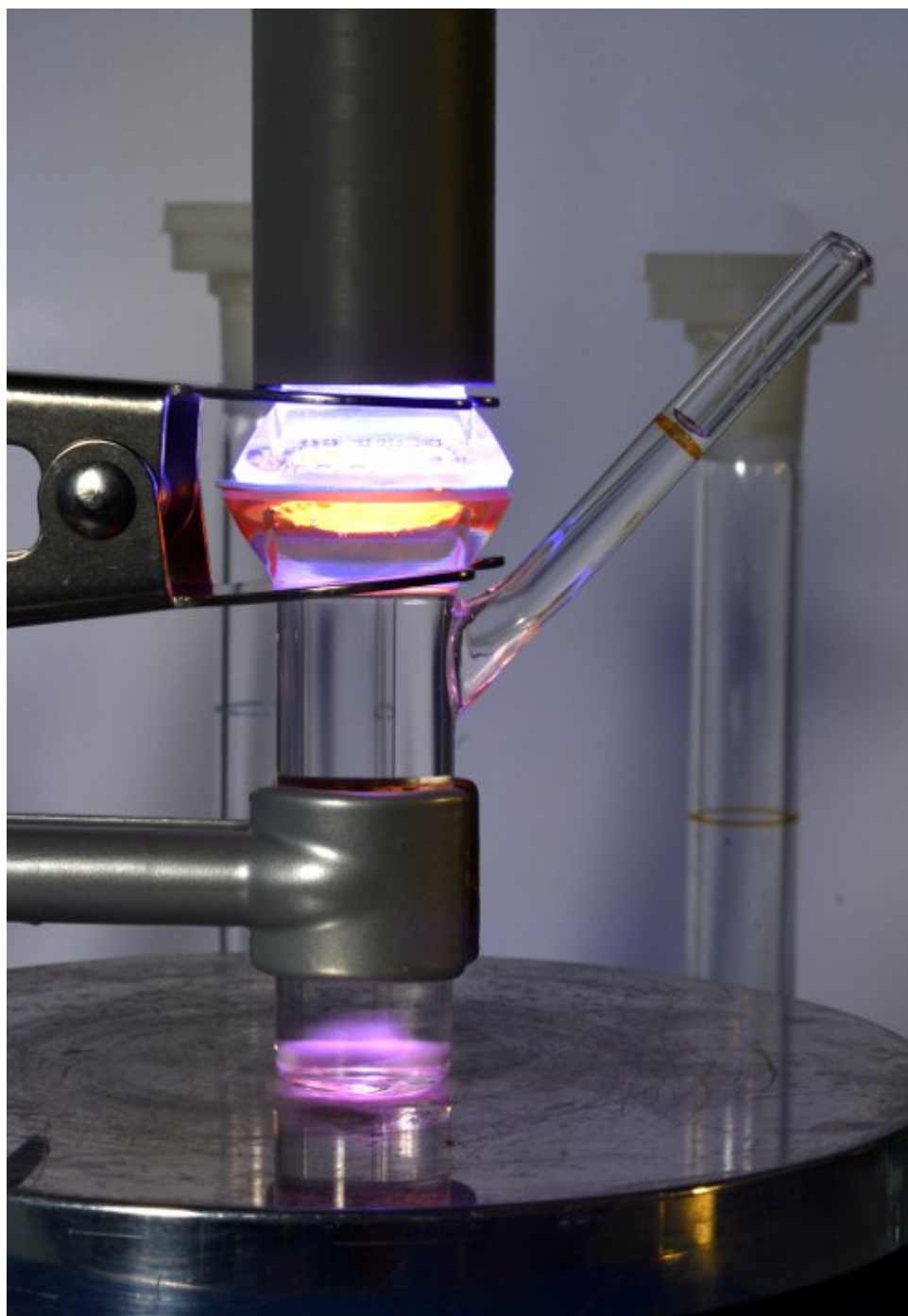
Figure 3. The Franz diffusion cell with the fixed membrane between the receptor chamber (bottom) and the donor chamber (top). The light source is fixed on top of the Franz diffusion cell (here: UV light).
