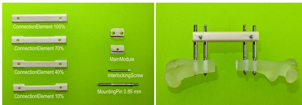
Figure 7. Components of the external fixators. Left: Stiffness is determined by connection elements of different thicknesses. The fixator is attached to the bone with titanium alloy mounting pins. Right: Assembled fixator in place on rat femur with 5 mm segmental defect.
