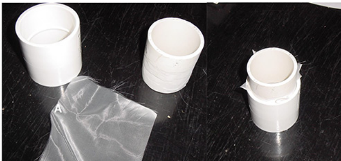
Figure 2. Construction of sieve to separate scale eggs from adults and other contaminants. A 4 x 4 inch pre-cut square of 250 micron nylon mesh is placed between a 4 inch piece of 2" diameter PVC pipe and a coupling to form the sieve.
