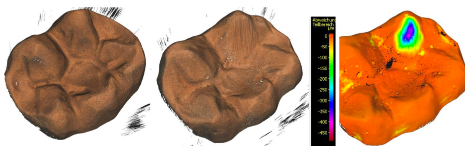
Figure 21: Difference image between a test specimen before and after chewing simulation, color graded from -20 \mu\text{m} (orange) to -500 \mu\text{m} (purple). The high-resolution scan of the tooth surface is used to evaluate the abrasion of different restorative materials with in vivo and in vitro tests. Click here to view larger image.
