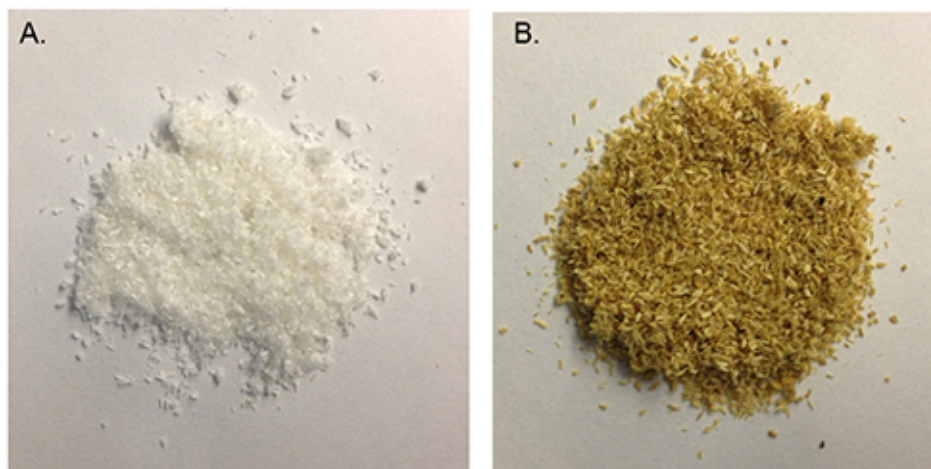
Figure 5. Comparison of bleaching methods. A) Dried hollocellulose using \text{NaClO}_2 bleaching. B) dried hollocellulose using \text{NaOH} bleaching. Comparison of color indicates increased delignification when \text{NaClO}_2 is used as a bleaching agent. Click here to view larger image.
